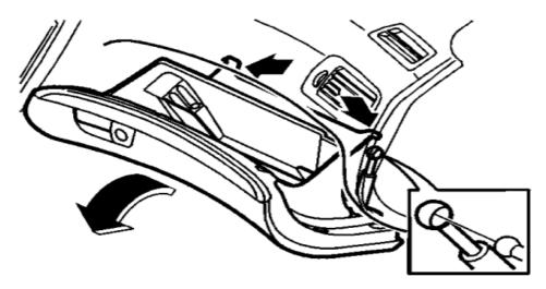
• Slide the two hooks on each side past the tabs. Remove the gas strut by pulling it straight out.
